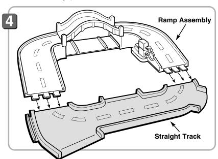
• Insert and "snap" the tabs on the end of each ramp into the slots in the straight track as shown.
